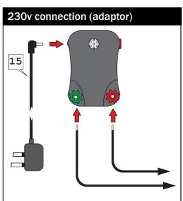
Mount the energiser next to an indoor socket. Insert the male jack of the adaptor into the socket and plug in the adaptor head. Connect the HT lead for your fence and ground connections to the terminals (HT is not included in the pack as power to fence distance varies).
