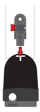
Push the bracket tab into the top of the energiser ensuring a tight fit
